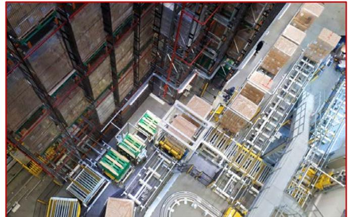
All the pallets are labeled with a bar code and transported inside the automated warehouse through an RGV shuttles system. The RGVs move within a closed circuit and are used both for the supply of the warehouse, at the entrance, and for the picking, at the exit.
